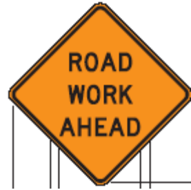
Sample ROAD WORK AHEAD Warning Sign (Source: MUTCD)
